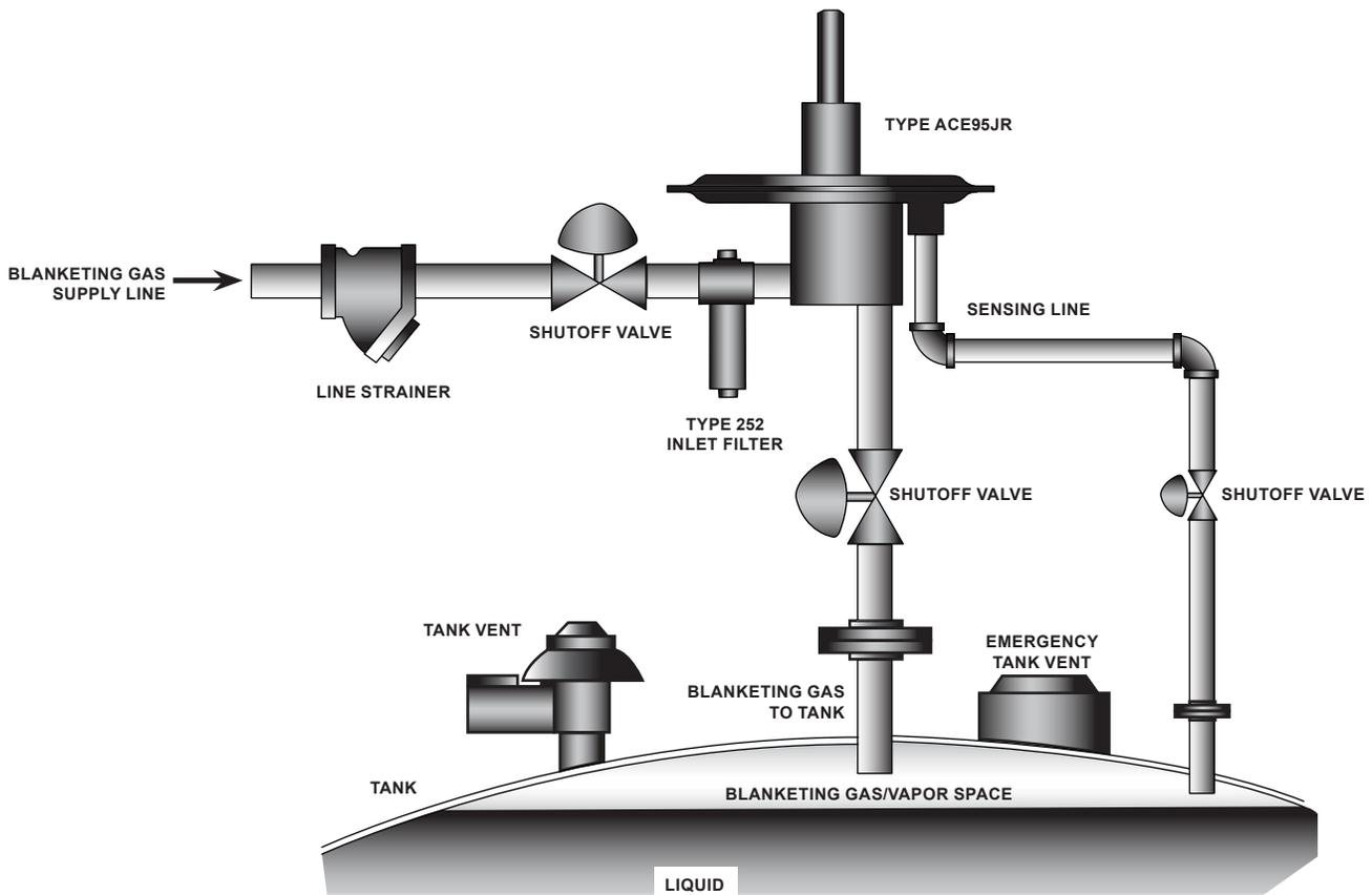
Figure 3. Type ACE95jr Tank Blanketing Valve Installation
